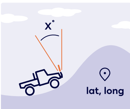
Inbuilt GPS and gyroscope detect antenna location and attitude (tilt)
